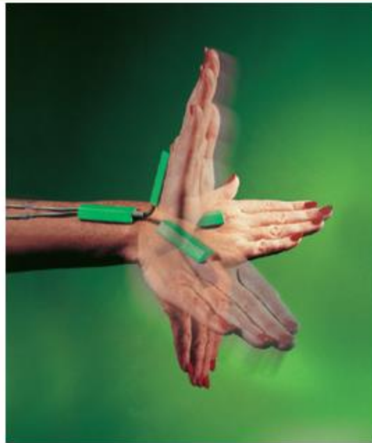
FIGURE 4-24. A biaxial electrogoniometer measuring wrist flexion and extension as well as radial and ulnar deviation. (Courtesy Biometrics, Ltd, Ladysmith, Virginia.)
