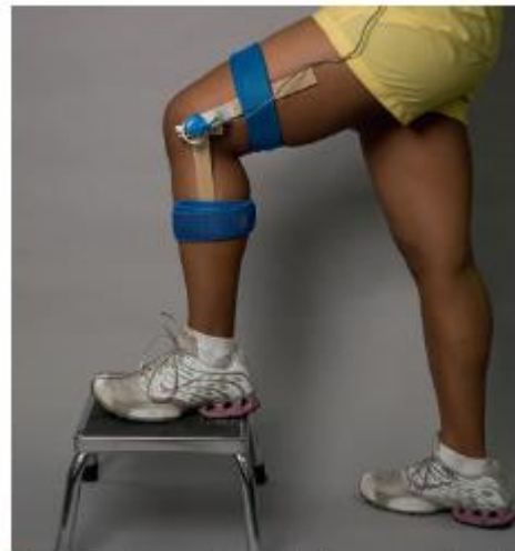
FIGURE 4-23. An electrogoniometer is shown strapped to the thigh and leg. The axis of the goniometer contains the potentiometer and is aligned over the medial-lateral axis of rotation at the knee joint. This particular instrument records a single plane of motion of the knee only.
